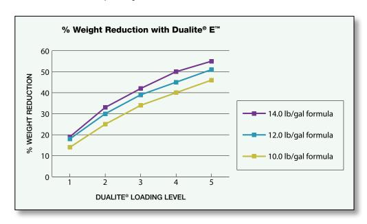
The chart demonstrates the percent weight reduction for formulas with initial specific gravities of 10, 12, and 14 pounds/gallon at different loading levels of Dualite® E065-135D™.
