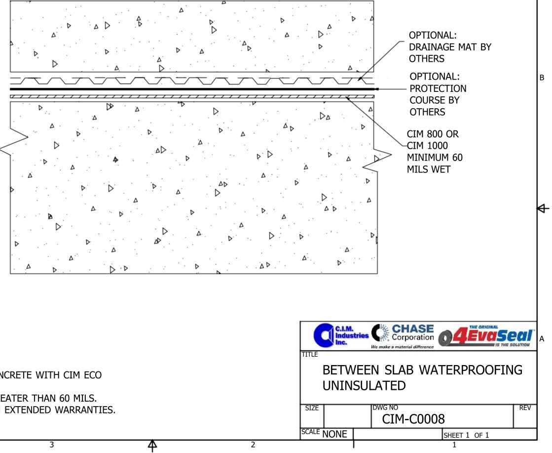
NOTES: 1. (OPTIONAL/NOT SHOWN) PREIME CONCRETE WITH CIM ECO OR CIM EMT EPOXY PRIMER. 2. MAY BE APPLIED AT THICKNESSES GREATER THAN 60 MILS. CONTACT CIM FOR INFORMATION ON EXTENDED WARRANTIES.
