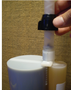
4. Static Mixer Attached to Cartridge With Retaining Nut
